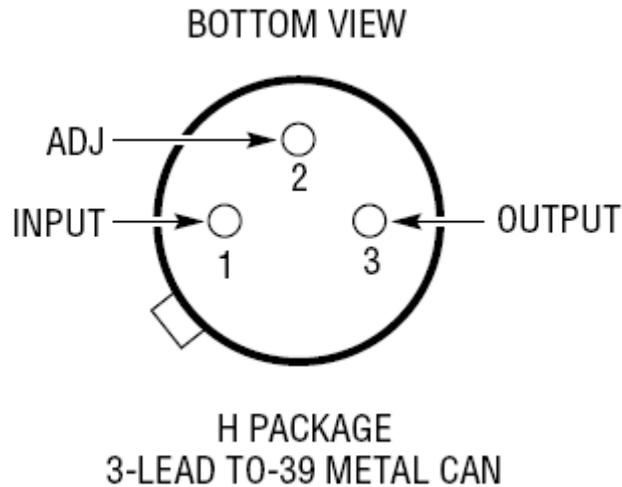
Figure B.2. H package drawing (for reference only). This figure was extracted from the LINEAR TECHNOLOGY CORPORATION RH117 Datasheet.
